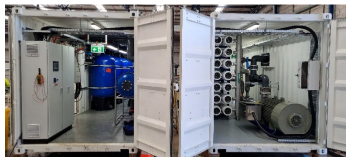
Internal view of the containerised SWRO and pre-filtration & control containers in the MAK Water factory
